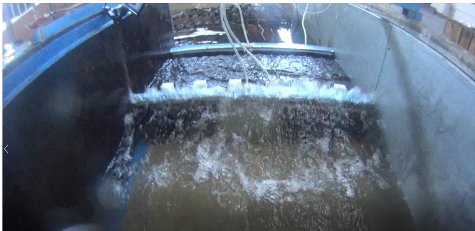
Figure 5.16: During the experiment of setup 4 wave 5 ( H_{s0} = 0.088\text{m} and T_m - 1,0 = 1.37\text{s} )
