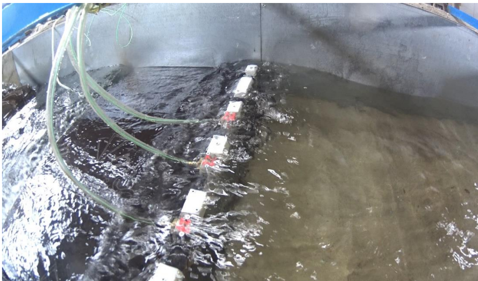
Figure 5.4: During the experiment of setup 1 wave 1 ( H_{s0} = 0.081\text{m} and T_{m-1,0} = 1.26\text{s} )
