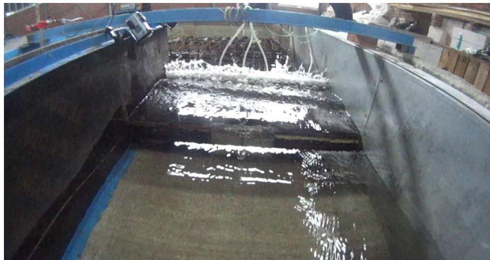
Figure 5.18: During the experiment of setup 7 wave 5 ( H_{s0} = 0.088\text{m} and T_{m-1,0} = 1.37\text{s} )
