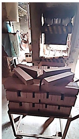
Figure 4.11. Facing refractory bricks produced from compression molding machine
