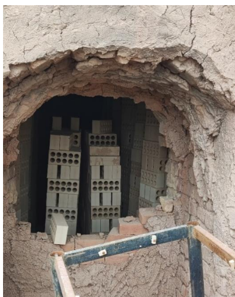
Figure 4.16. Stacked hollow clay bricks in kiln
