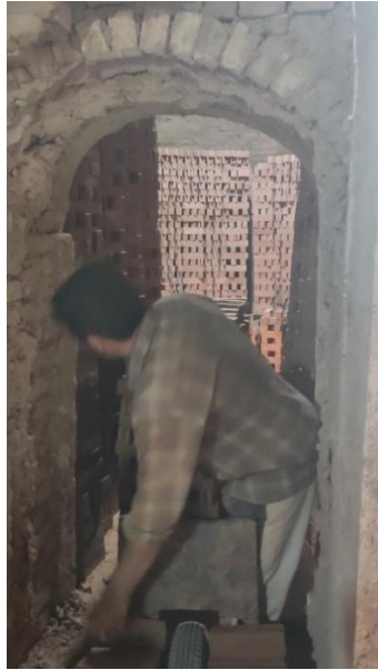
Figure 4.17. Arrangement of red clay bricks in the kiln
