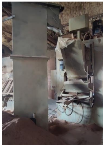
Figure 4.9. Lifting system for transferring grinded and moist soil to the molding machine
