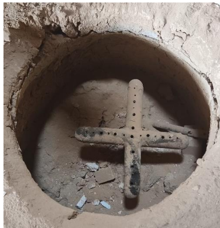
Figure 4.18. Gas burner in the center of the kiln.
