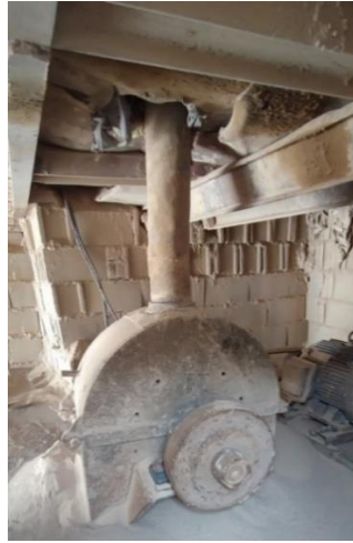
Figure 4.5. Third type of Grinding systems with 40 hp electric motor
