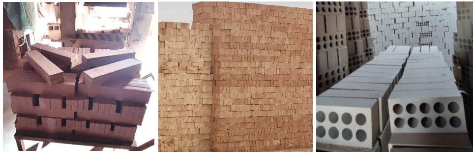
Figure 3.1. Photos taken of refractory bricks (left), red clay bricks (middle), and hollow clay bricks (right), produced in the factory
