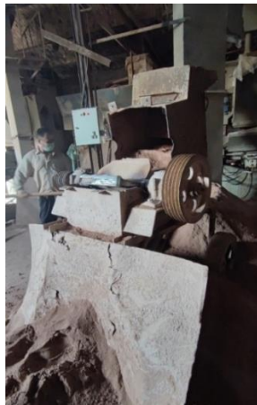
Figure 4.8. Mixer and soil homogenizer system
