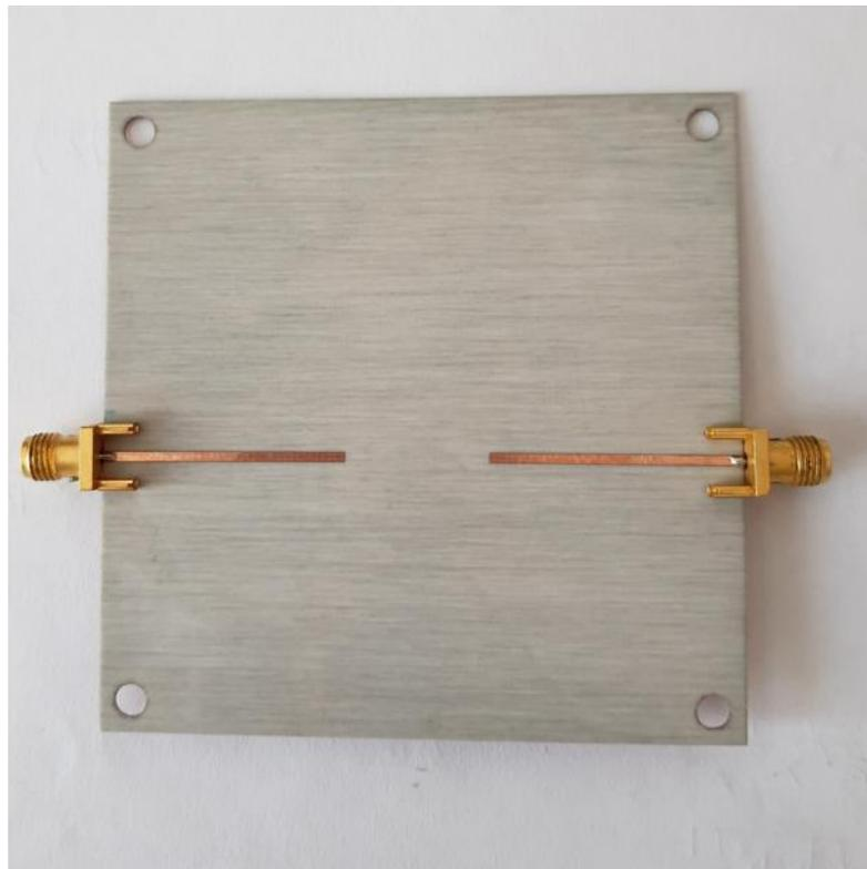
Figure 5.23: Antenna feeding with two microstrip lines
