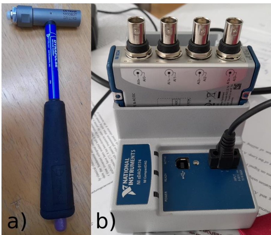
Figure 2.5 a) Hammer Used for Tap Tests. b) NI 9234 Data Acquisition Device Allows 4 BNC Ports That Measures Voltage Difference
