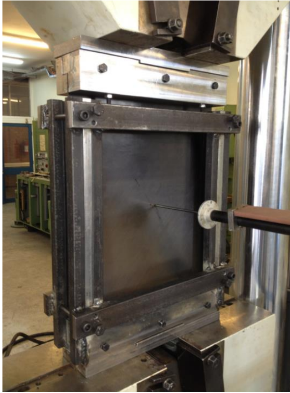
Figure 5.2. Experimental Setup of Constant Stiffness Plate
