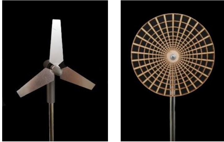
Figure 2.2. Models used in wake measurements: the model wind turbine (left) and the porous disc (right).
