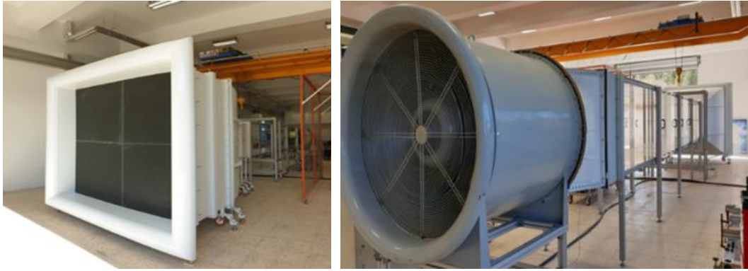
Figure 2.1. The open-return suction type boundary layer wind tunnel is utilized for the wake measurements.
