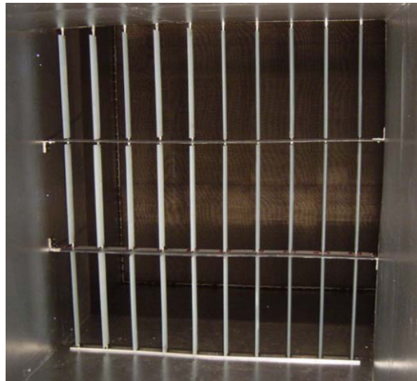
Figure 1.9: Disturbance generator mounted in the wind tunnel contraction in Virginia Tech Stability Wind Tunnel [30].
