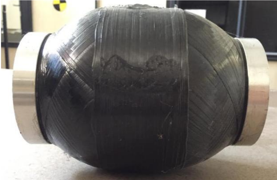
Figure 3.27 Composite pressure vessel manufactured that is to be subjected to impact hammer modal test
