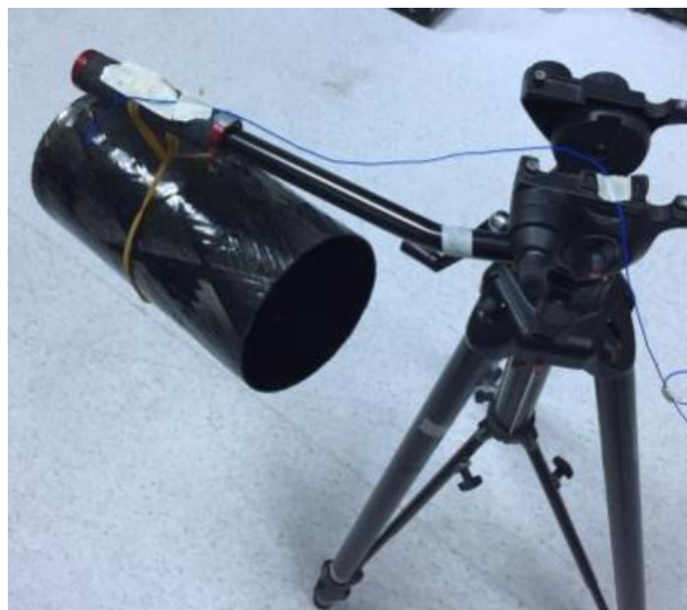
Figure 3.26 Composite cylinder subjected to impact hammer modal test
