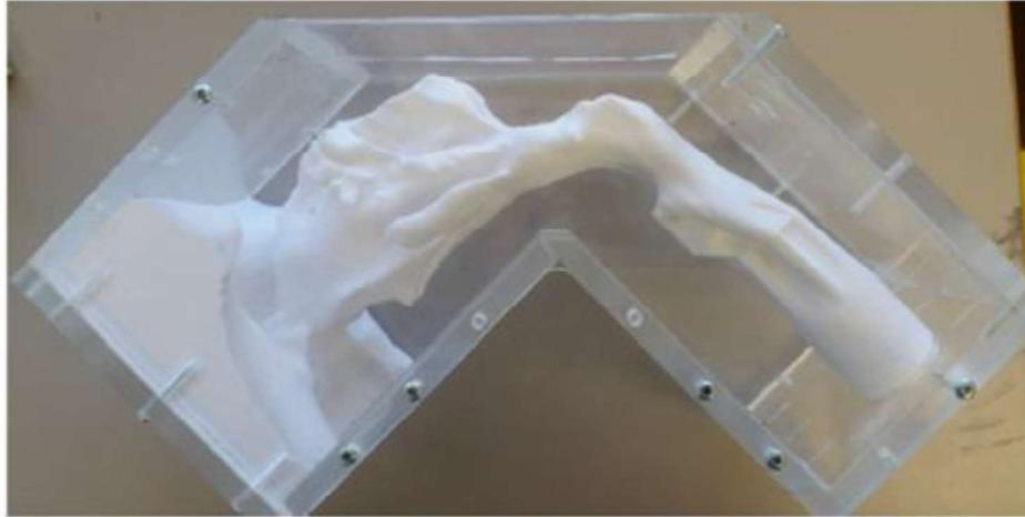
Figure 2.8. Lost-core casting- the casting box's surfaces are arranged in a way to increase optical access to vital areas [20]
