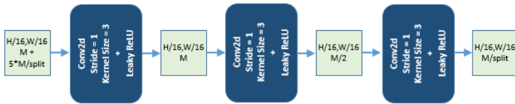
Figure 4.9: Latent residual prediction network
