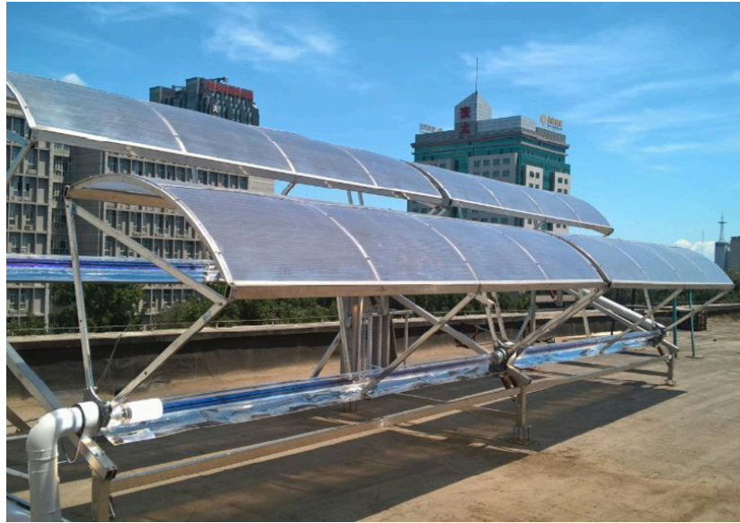
Figure 1.10: Experimental setup of a cylindrical Fresnel solar collector system, Ma et al. [34].
