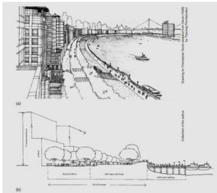
Figure 3.36. The Shanghai waterfront Proposal (a) sketch of the proposed crescent and (b) a cross section through the crescent (Lang, 2005, p.110).
