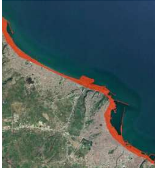
Figure 4.12. Comparison of the growth in the city's coastline due to the fill areas from 1950 to 2022 (Edited by the author).
