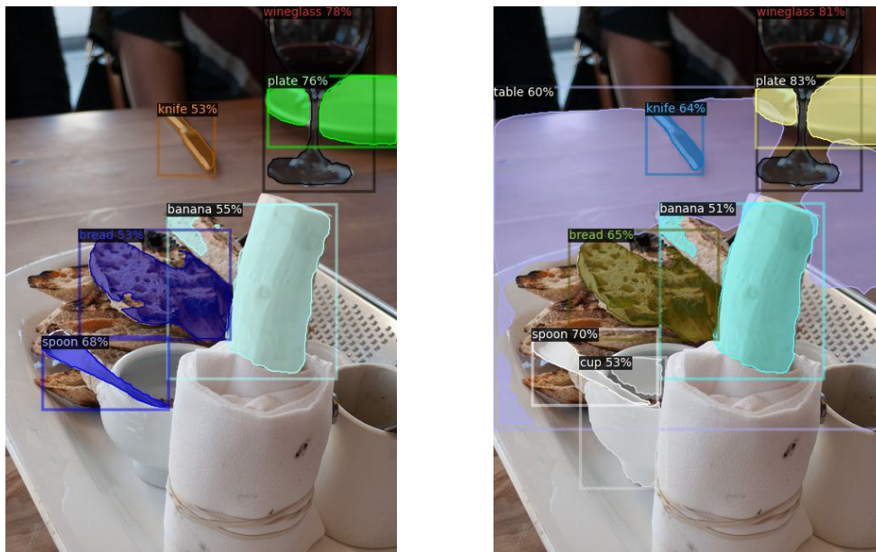
Figure 4.2: Comparison between RFS baseline [17] (left) and PriorBox (right). PriorBox predicts higher probabilities for true positives (wineglass, knife, plate, bread and spoon), detects more ground truths (table and cup) and gives less confidence to false-positives (banana) than the baseline. Image is picked from LVIS v1 validation split.
