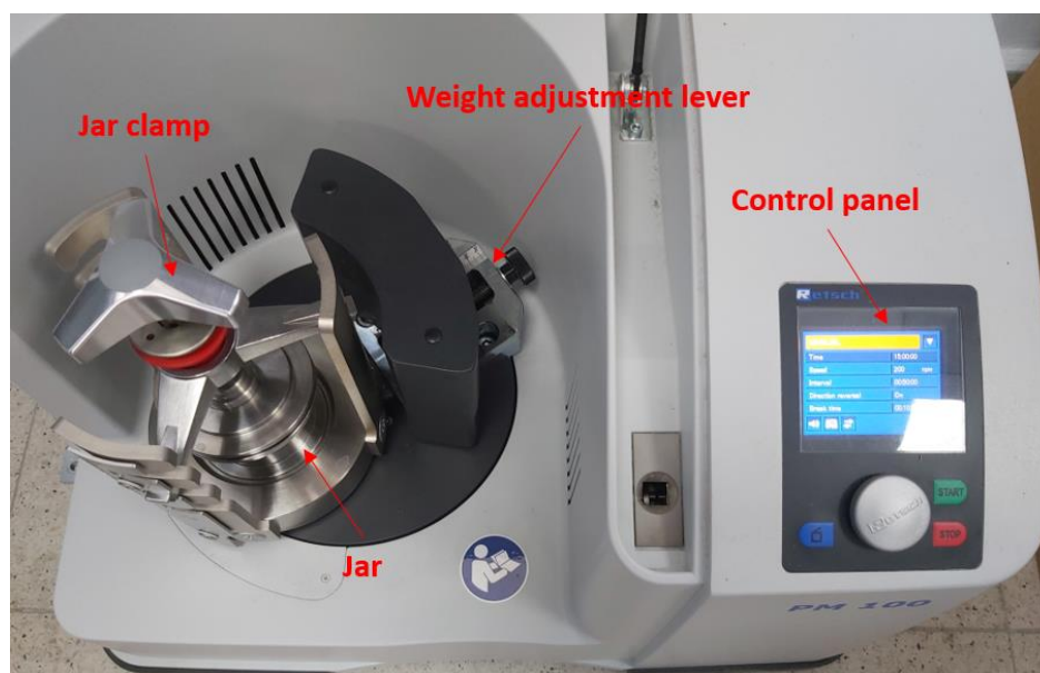
Figure 2.2 Photograph of ball-milling device.
