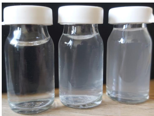
Figure 3.8. Photo of shear exfoliated samples (sorted from left to right as for once, twice and three times).
