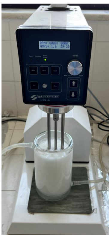
Figure 2.1. Photograph of shear exfoliation device.
