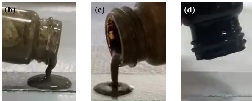
Figure 6.13. (a) The rheological behavior of aqueous suspensions of Sample D, Sample E and their comparison with the one of the reference powders. The images showing the flow behavior of the suspensions prepared from (b) the Sample D, (c) the Sample E, and (d) the reference powder.
