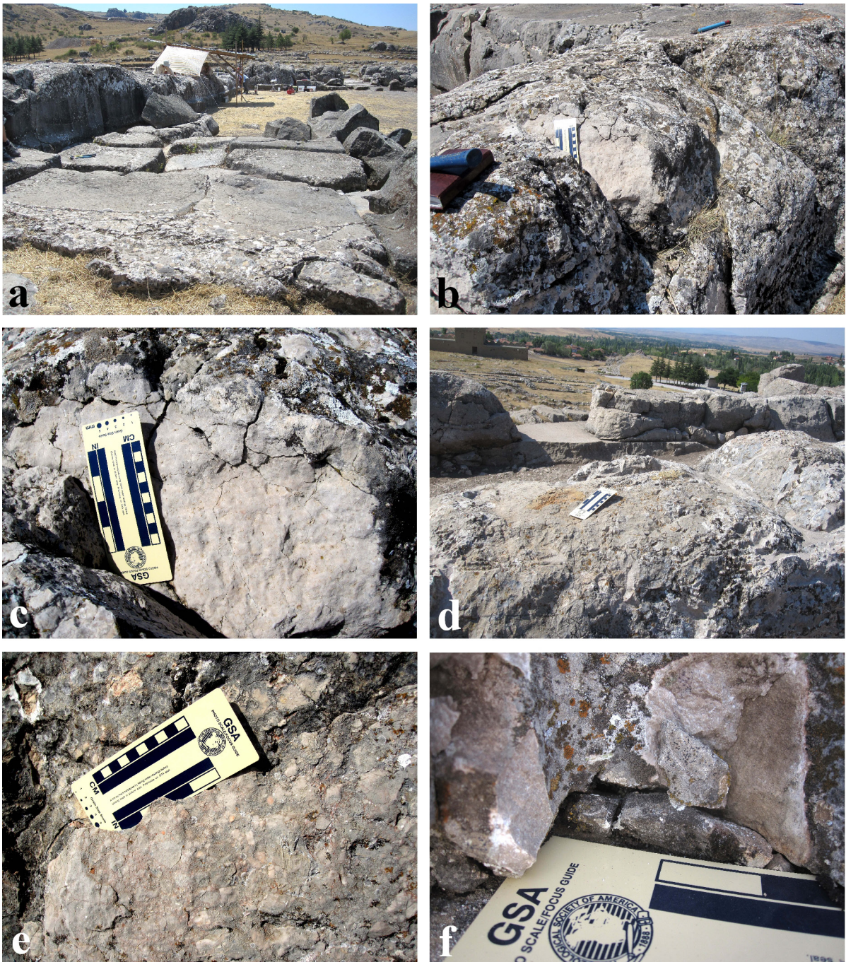
Figure 5. Field photographs of the wall blocks of the Great temple, a) general view of the thick-very thick bedded limestone blocks along the wall (looking towards west), b) limestone block with bioclastic facies (sample 210), c) close up view of b, d) limestone block with breccia facies including intrclasts (sample 157), e) limestone block with intralcast and fossils (sample 167), f) Limestone block with pelloidal, intraclastic facies (sample 31).
