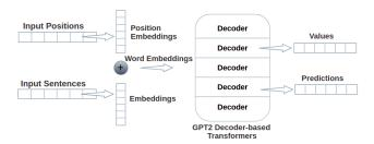
FIGURE 4: GPT2-DSLM and GPT2-GLM based on GPT-2 architecture
