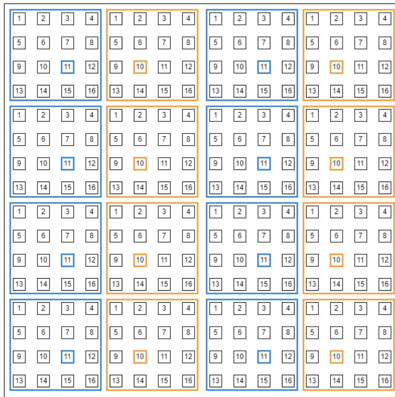
Figure 4.35. A 16 \times 16 array antenna with 4 \times 4 calibration sub-arrays
