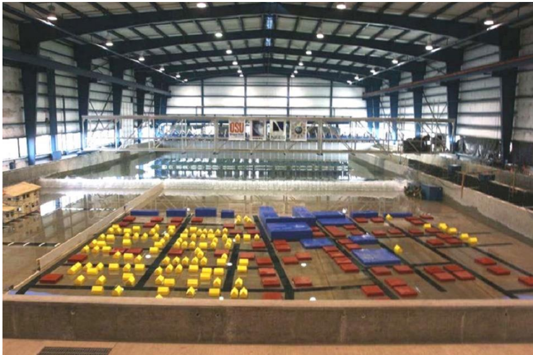
Figure 4.17 The physical model of Seaside, Oregon (Cox et al., 2008; Rueben et al., 2011).
