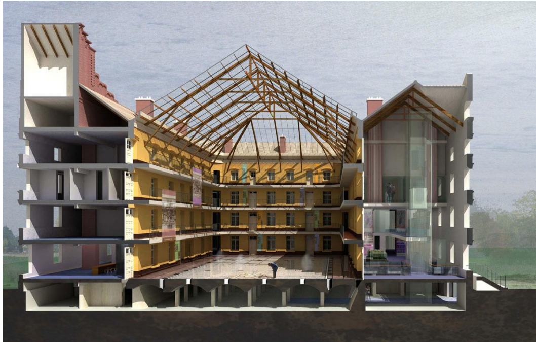
Figure 2.7 Cross-section of the central pavilion of the Familistère de Guise. Frenak + Jullien architects, 2006. Source: familistere.com
