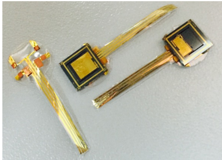
Figure 3.9. Parylene attachment layer with metal connection lines and copper spacer columns. Two chips from the SOI-2 wafer were bonded using epoxy on the copper columns.
