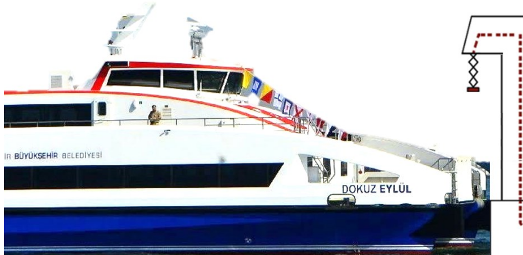
Figure 3.11. Bow-type chargers are ideal for charging passenger ferries in İzmir.
