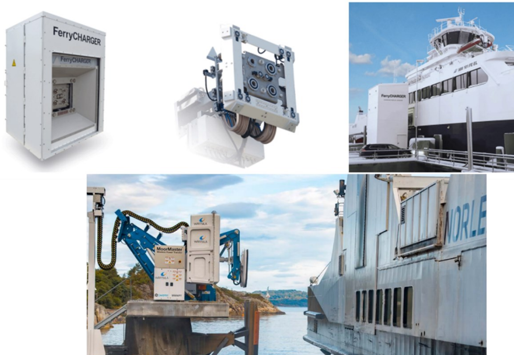
Figure 3.9. Examples of different methods for transferring power from shore ESS to ferry ESS. Top row: Plugged power transfer system. Bottom row: Wireless power transfer system. Photos from [60].
