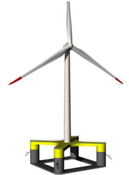
Figure 9 Nautilus DTU-10 FOWT concept (Galván, Sanchez-Lara, et al., 2018)
